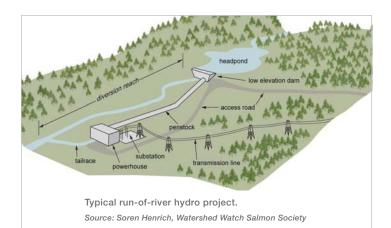
Some hydro projects use a dam to store water, while others divert water from the river flow without significant storage. Hydro projects without significant storage are often known as 'run-of-river.' Note that even run-of-river projects may involve small dams, in order to keep the penstock submerged. The definition of run-of-river is based on the amount of water stored behind the dam or weir, usually defined as less than 48 hours of storage capacity.
